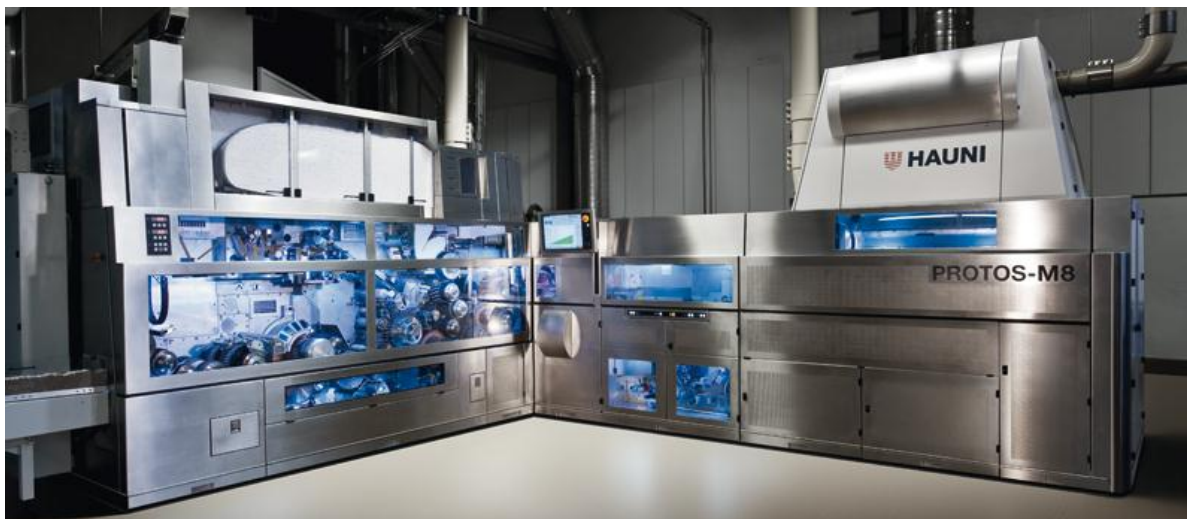
Figure 1: Machine fabriquant des cigarettes (Hauni Protos M8)
